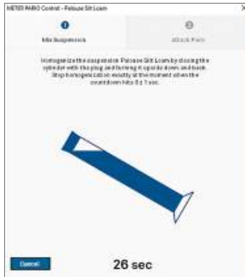
Figure 6 PARIO Control homogenization countdown with mixing instructions
