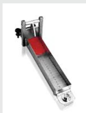
As the fluid flows down the instrument its progress can be accurately measured using the graduated scale. By comparing the flow rate to specified time periods the physical properties of the sample can be calculated.
