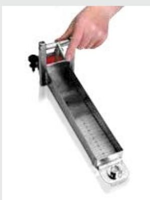
The gate is released by pressing the lock release lever - the spring action ensures it opens instantaneously.
