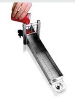
A measured sample up to 100 ml is placed in the reservoir behind the gate.
