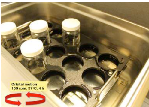
Figure 5. Grant OLS 200 ® shaking incubation bath set at 37°C showing custom made polypropylene holder for Fisherbrand ® 250 mL bottles.
